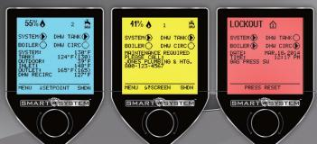
Blue Screen Normal system operation Yellow Screen Maintenance due shows installer name & number Red Screen Lockout mode
