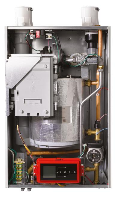
CTRLMAX Control System -EZ Setup allows for quick 60 second setup. Easy troubleshooting in plain text, no codes. Stainless Fire Tube Heat Exchanger. 3 in 1 Universal vent adapter directly accepts PVC, Polypropylene, Stainless steel. Large plate heat exchanger provides industry leading performance. 5+ GPM hot water while fully condensing in DHW mode.
