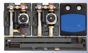
The ThermalPro<sup>™</sup> boiler connection station is a modular, compact, pre-piped mechanical system complete with circulator, isolation ball valves, thermometers, pressure bypass valve and, on mixed stations, a 24 volt, 3-way mixing valve.
